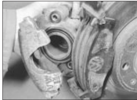
2.3b Removing the caliper
