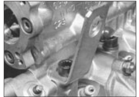
5.23 Engine lifting eye
