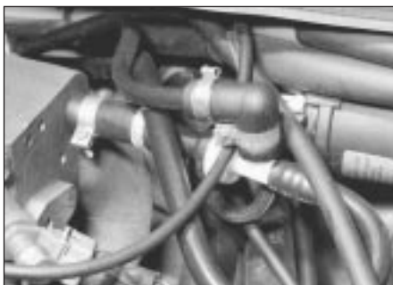
23.5 Vacuum hose-to-cylinder connector
