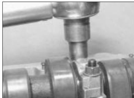
10.5 Tightening a camshaft bearing cap nut
