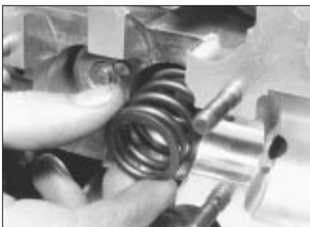
5.11a Removing an outer valve spring
