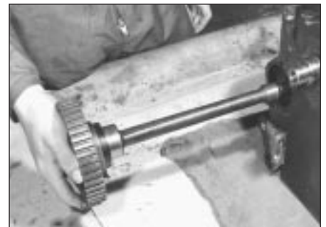
16.5b Withdrawing intermediate shaft
