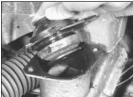
8.1a Lift the mounting away
