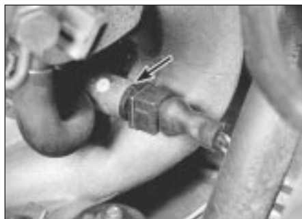
10.3 Auxiliary air valve (arrowed)
