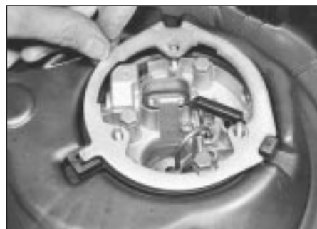
3.2 Removing air cleaner body retaining ring - 1.3 litre
