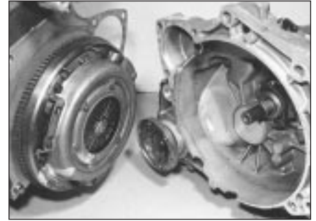
6.6b . . . then separate engine and transmission
