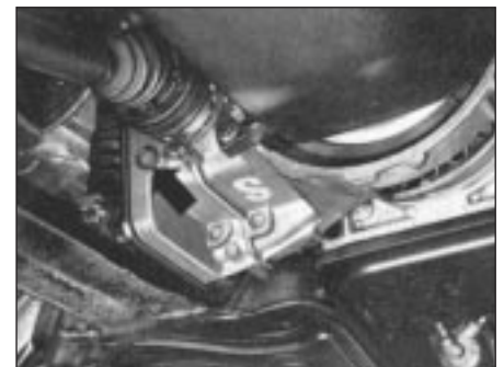
35.10 Final drive unit oil filler/level plug (arrowed)
