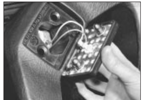
11.3a Removing steering wheel centre cover - 1.3 litre
