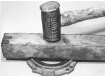
14.16 Installing new crankshaft rear oil seal
