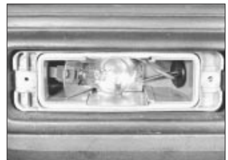
8.5 Front indicator lamp bulb
