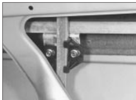
20.3b Lifting plate-to-window channel bolts
