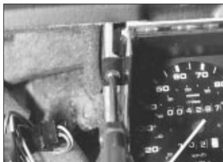
16.3 Instrument panel screw removal
