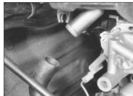
3.3b ... and crankcase emission hose - 1.3 litre
