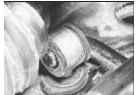
4.5 Anti-roll bar location in eye bolt
