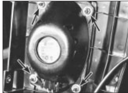
32.5 Luggage compartment loudspeaker retaining nuts (arrowed)
