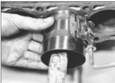
30.4 Using a piston ring compressor
