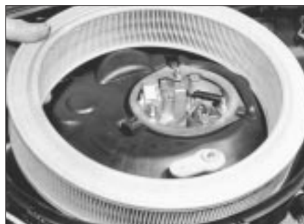
32.2 . . . and remove the element - 1.3 litre, carburettor
