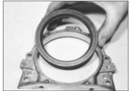
14.14 Remove crankshaft rear oil seal from housing
