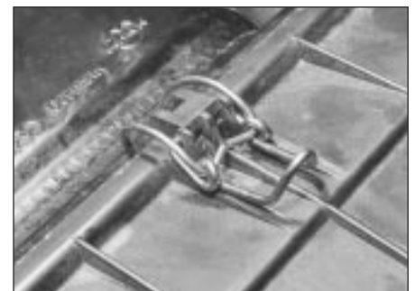
32.4a Unclip air cleaner cover . . .
