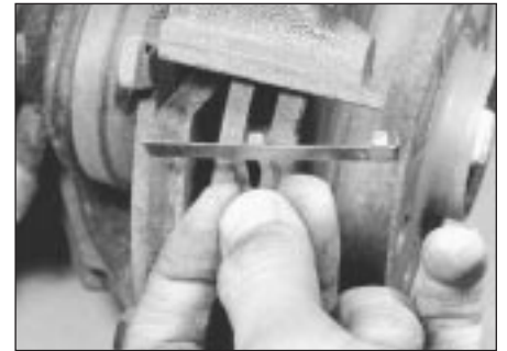
2.5 Removing a pad retaining spring
