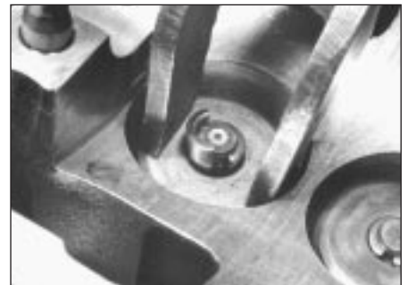
12.12c . . . and valve collets
