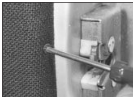
14.7b Trim panel retaining screw removal (rear edge)
