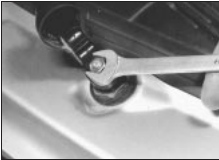
26.2 Undo wiper arm nut . . .
