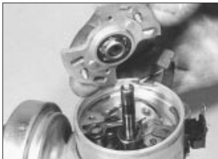
16.3 Removing the bearing plate - 1.05 and 1.3 litre
