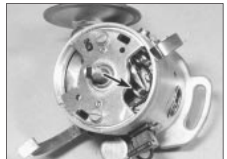
11.4 Contact breaker points viewed through window in bearing plate (arrowed) - Ducellier
