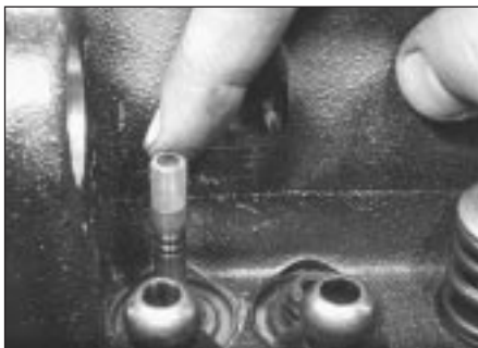
34.3 Locate plastic sleeve on valve stem . . .
