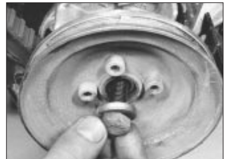
12.7 Removing crankshaft sprocket bolt and washer
