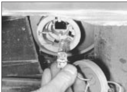
7.2 Bulb and holder removal from foglight
