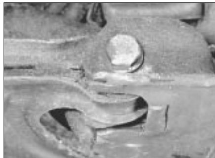
7.4 Track control arm pivot bolt
