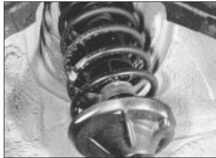
29.4 Check shock absorbers for leakage
