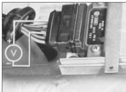
5.4 Voltmeter connection when testing Hall sender
