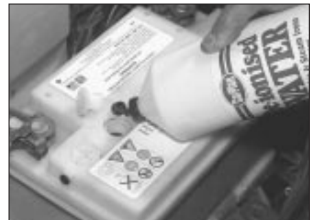
7.3b . . . and top up electrolyte level using distilled or de-ionised water
