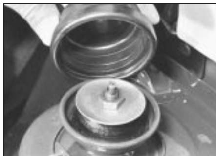
8.4 Removing rear suspension strut top cap
