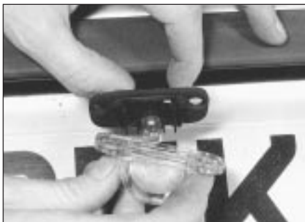
8.10 Number plate lens removal
