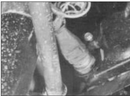
3.3a Radiator thermo-switch - 1.8 litre
