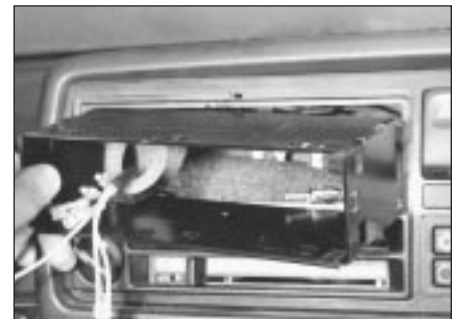
31.6 Radio/cassette container removal
