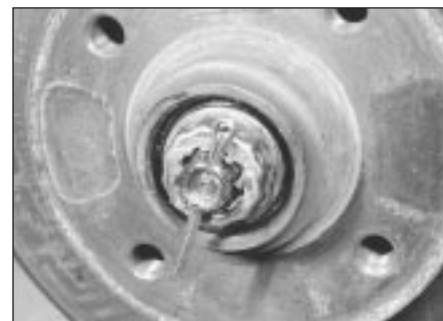
4.14 . . . remove the split pin and lock ring . . .
