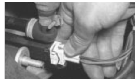
E Wiring plugs may cause problems if dirty or not connected properly.
