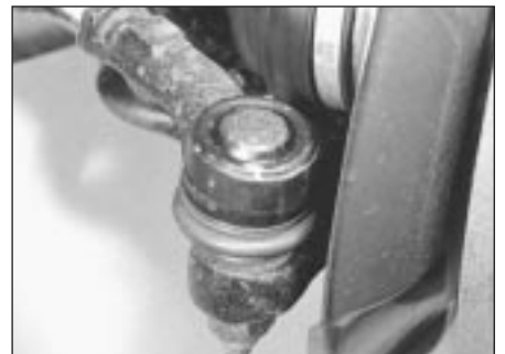
28.2 Inspect balljoint dust covers
