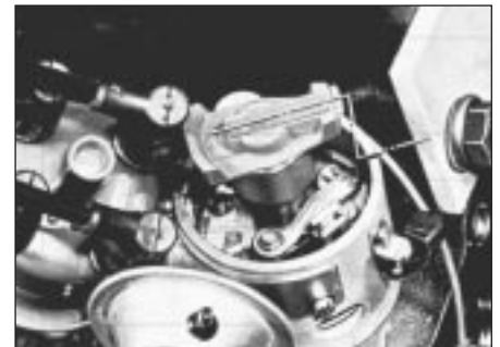
17.3c Rotor arm aligned with TDC mark on distributor body - 1.6 and 1.8 litre
