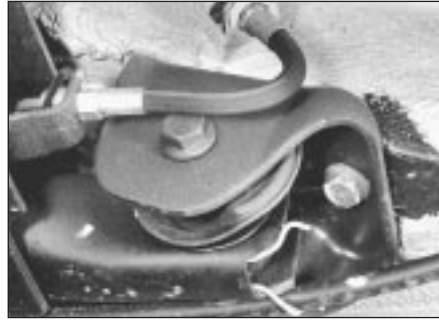
9.7 Axle beam pivot bolt head fitting position
