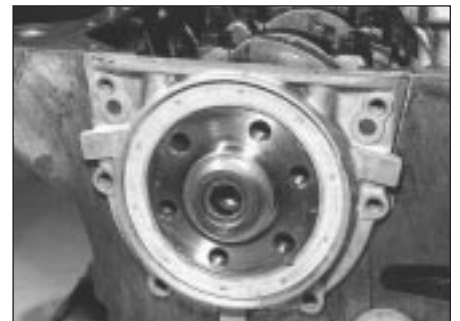
30.9 Fitting crankshaft rear oil seal and flange
