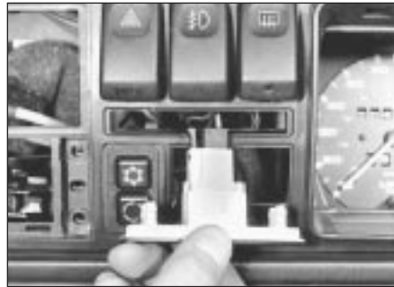
10.2 Warning lamp cluster removal
