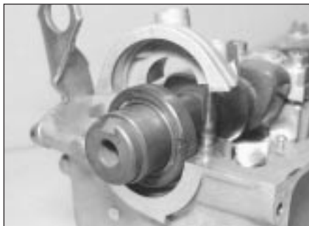
10.3 Camshaft oil seal
