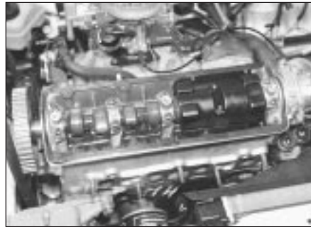
11.17 Plastic oil shield correctly located
