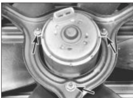
4.4 Cooling fan motor retaining nuts (arrowed)
