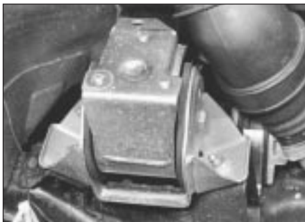
8.1b Right-hand rear mounting viewed from above
