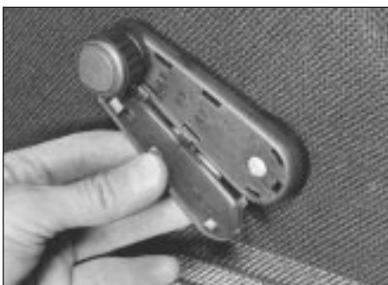
14.4a Remove window regulator handle cover . . .
