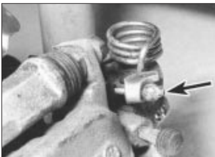
2.15 Release handbrake cable (arrowed) from caliper
