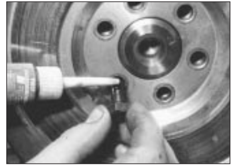
33.3 Applying liquid locking fluid to flywheel bolts
