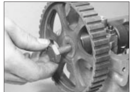
10.8 Fitting the camshaft sprocket bolt
