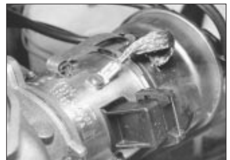
11.10 Fitting distributor cap and earth lead
