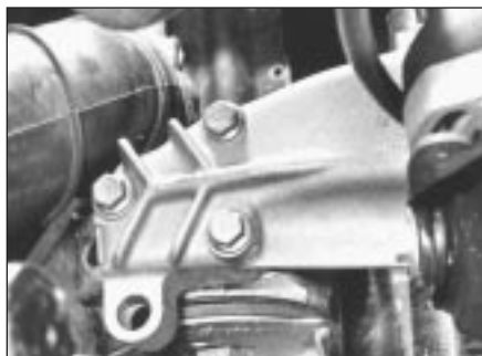
5.24 Engine mounting/bearer - right-hand
