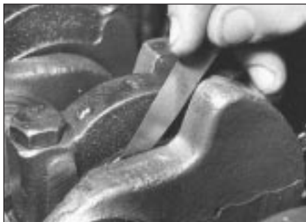
15.3 Checking crankshaft endfloat at No. 3 main bearing
