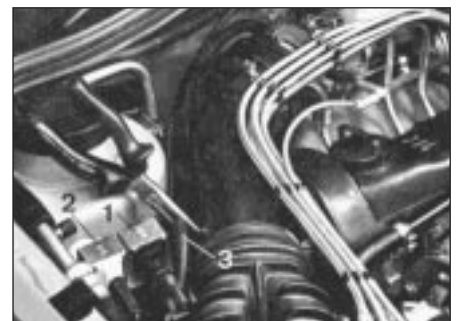
6.1 Idle speed boost valve check
