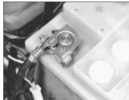
4.2 Battery positive terminal connection
