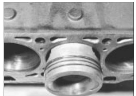
17.8 Removing a piston
