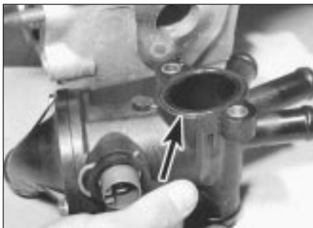
11.4 O-ring (arrowed) in thermostat housing
