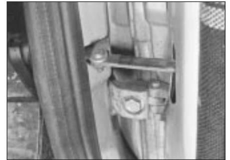
16.1 Door check strap and hinge
