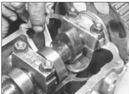
12.12 Removing a tappet bucket shim - 1.6 and 1.8 litre
