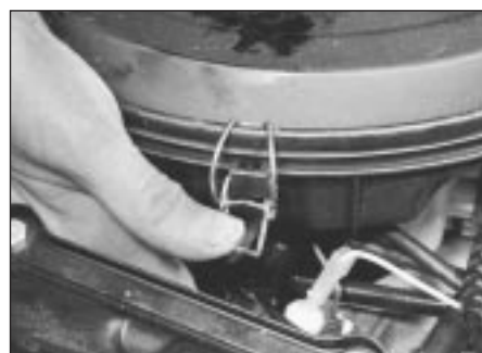
32.1 Unclip the air cleaner lid . . .
