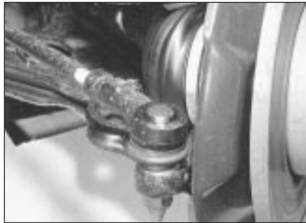
15.1 Right-hand adjustable balljoint
