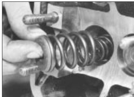
12.12b Locating valve springs and cap . . .
