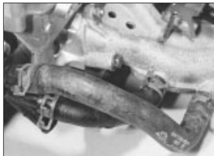
11.5 Coolant hoses in position
