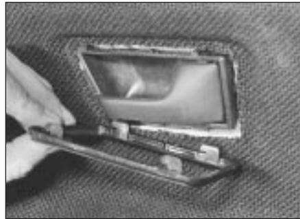
14.2 Removing door inner handle surround
