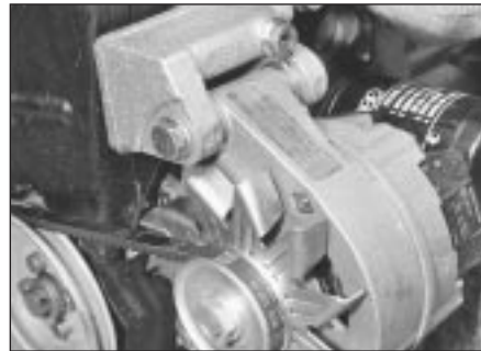
7.3 Alternator pivot bolt and bracket - 1.3 litre
