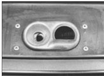
7.1 Bonnet lock and securing rivets
