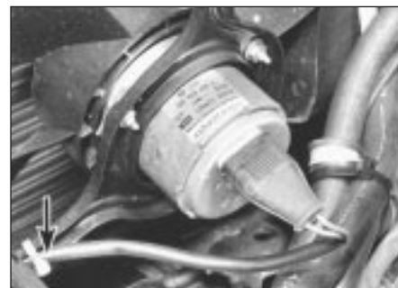
3.15 Secure fan lead with plastic clip (arrowed)
