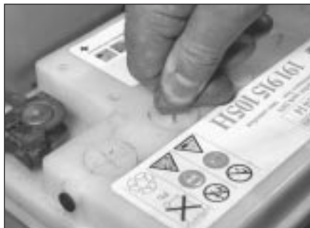
7.3a Remove battery filler caps . . .
