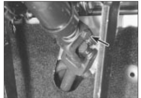
12.7 Steering column universal joint (upper). Clamp bolt arrowed
