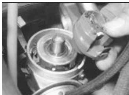
7.3a Pull free the rotor ...
