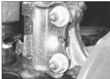
2.7 Strut-to-front wheel bearing housing retaining nuts/bolts
