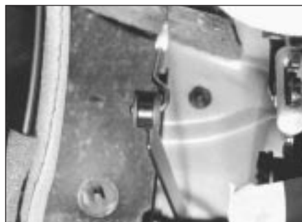
10.5 Accelerator cable-to-pedal attachment
