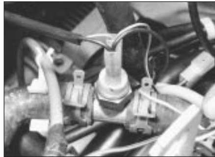
7.11 Temperature sender unit thermo-switch location - 1.05 and 1.3 litre
