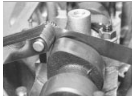
8.6 Measuring camshaft endfloat
