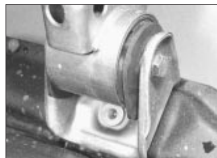
5.25a Engine/gearbox unit front mounting
