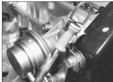
8.1c Engine dipstick and tube
