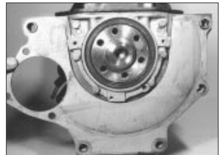
13.4 Removing engine plate
