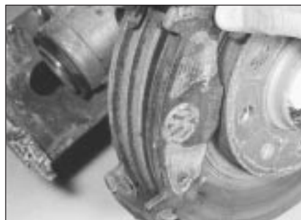
2.10 Refitting front brake pads
