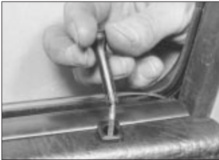
14.1 Unscrewing door locking knob
