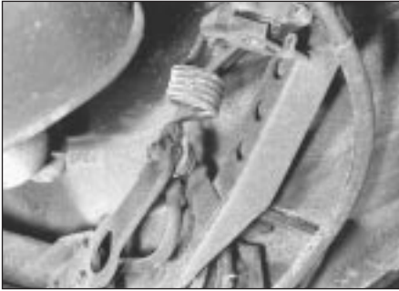
9.3 Brake pressure regulator unit showing spring bracket
