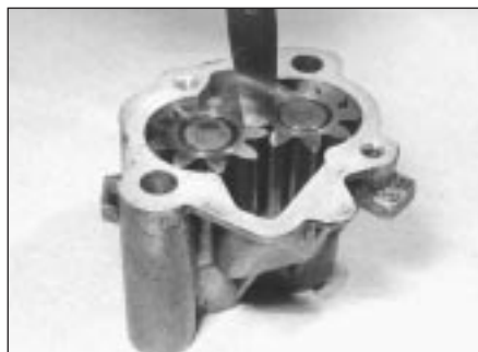
25.3 Checking oil pump gear backlash
