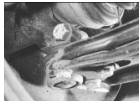
7.3 Track control arm balljoint and clamp bolt
