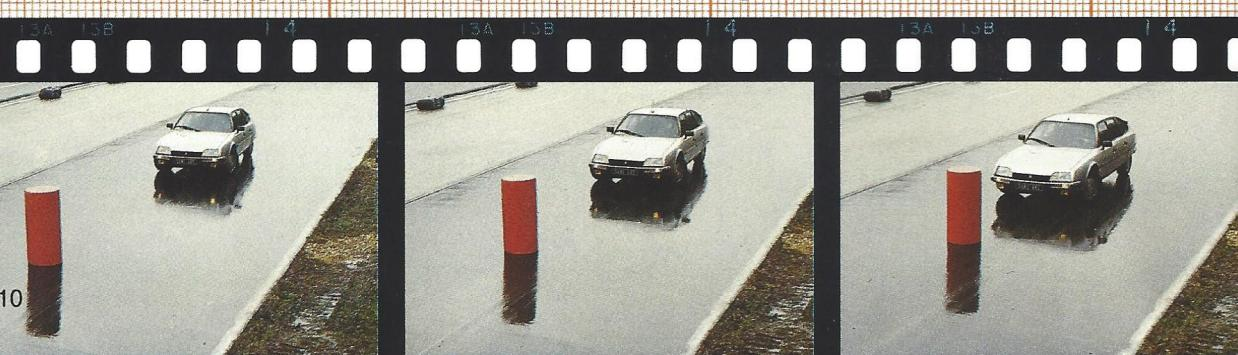
**The CX 25 GTI turbo is the first French car to be optionally equipped with the A.B.S system to prevent the wheels blocking when braking. Combined with hydropneumatic technique, this advanced technology is even more effective.**
