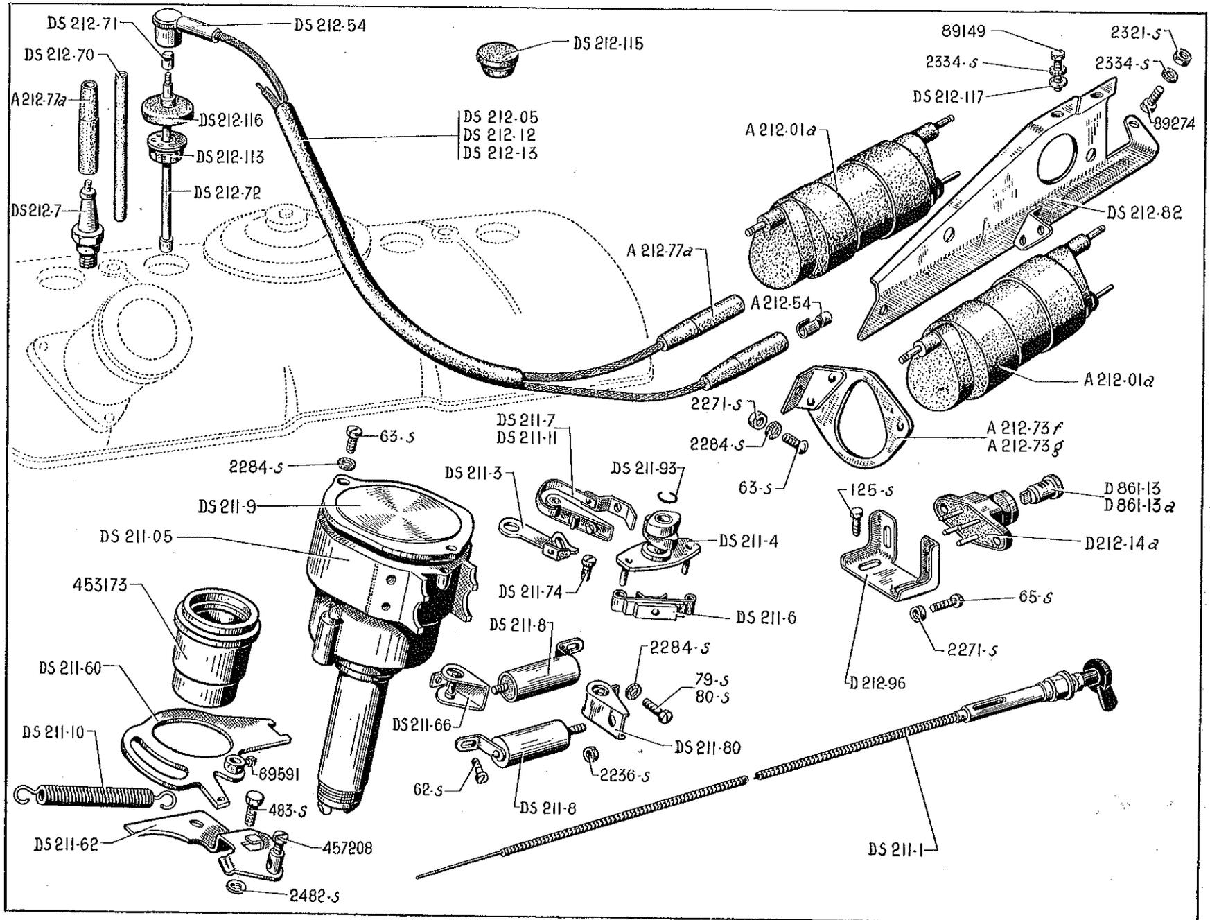
**ALLUMEUR ET BOBINE DUCELLIER - CIRCUIT D'ALLUMAGE - COMMANDE D'AVANCE (suite) — 29**
