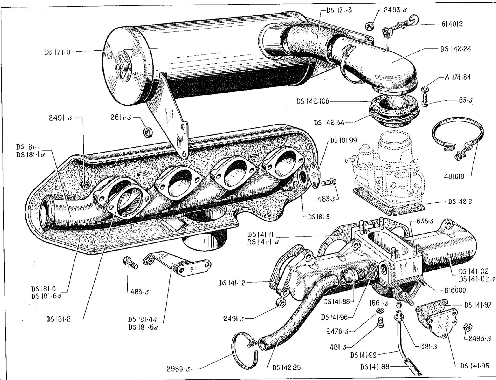
TUBULURES - CARBURATEUR - FILTRE A AIR — 9
